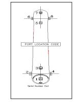
CODELINE BODY LABELS ARE PLACED AT 90° TO SERIAL NUMBER END AND AT 270° ON THE OPPOSITE SIDE END
