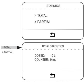
DOSED: total quantity dosed (max 999.999.999 L). COUNTER: water meter counter (cubic meter of water).
