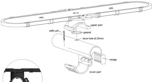
The hinge at the lower part of the clamp saddle is hooked into the upper part and the clamp saddle is closed around the pipe.
