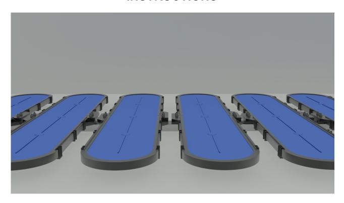
The OXYFLEX® - MF1100 membrane plate diffuser consists of a flat, heavily ribbed base plate with air-sockets. A two-piece frame secures the membrane to the base plate. The base plate and the frame are made from fibre glass-reinforced polypropylene, and the membrane is available in EPDM or TPU.
