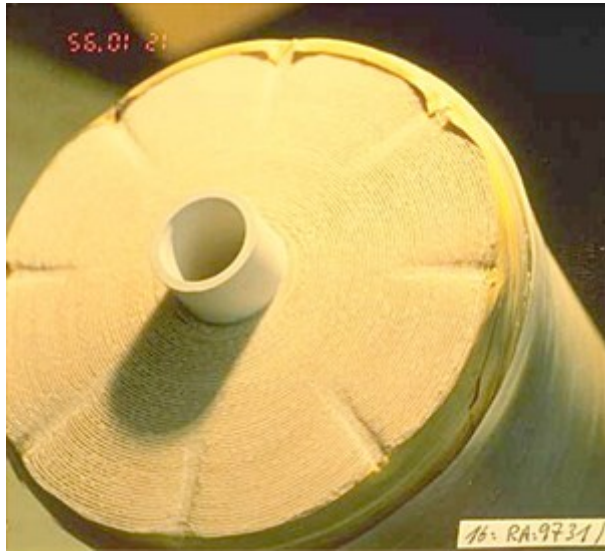
Figure 59. The endcap has been pushed off
