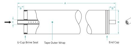
1. BW30 PRO-2540 Elements fit nominal 2.5-inch I.D. pressure vessel. BW30 PRO-4040 Elements fit nominal 4-inch I.D. pressure vessel.
